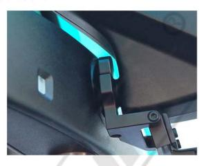
**STEP 6** - Rotate the mount so it is parallel with the bottom of the mirror. Tighten the clamp screw until the mount is securely attached to the mirror stem. Do not over tighten the clamp screw.
