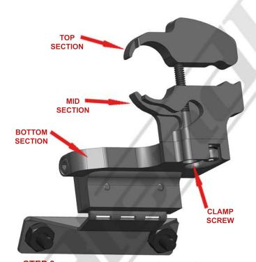
STEP 3 - Loosen the clamp screw so the top section seperates from the mid section. This will provide the necessary clearance to slide the mount over the mirror stem as shown above. Adjust the mirror parallel to the windshield and slightly upward for ease of installation.
