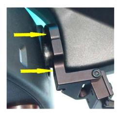
STEP 5 - Position the mount as far forward as you can. Tighten the clamp screw untill the Top and Mid Sections are slightly snug around the mirror stem. You should still be able to rotate the mount.
